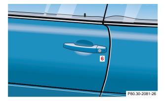
**6** Infrared receiver in driver's door handle
